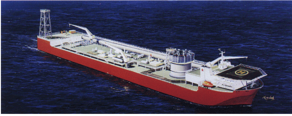
Figure 3: Moored ship: Length L = 200.6 (m) and mass m = 73.097.150 (kg).
