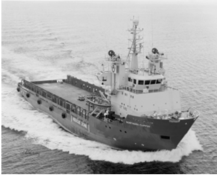
Figure 2.2: Supply vessel used in the North Sea. Length of ship: 76.2 m.
