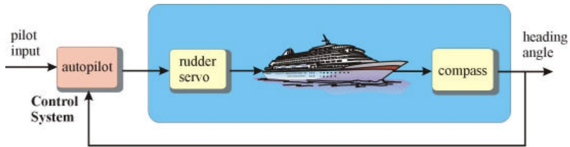
**Figure 1.** The conventional auto-pilot viewed as a feedback control system.
