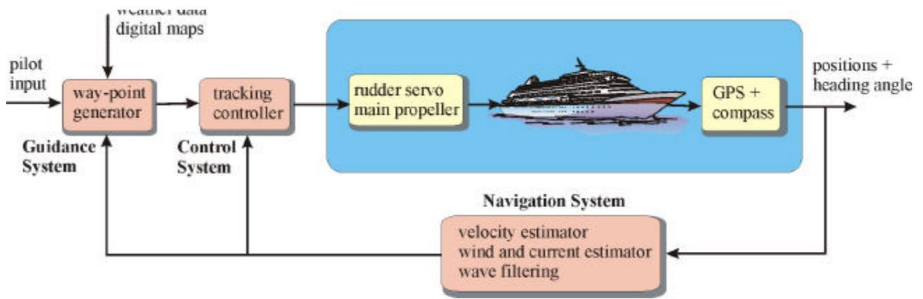
**Figure 2.** Guidance, navigation and control system for way-point tracking.
