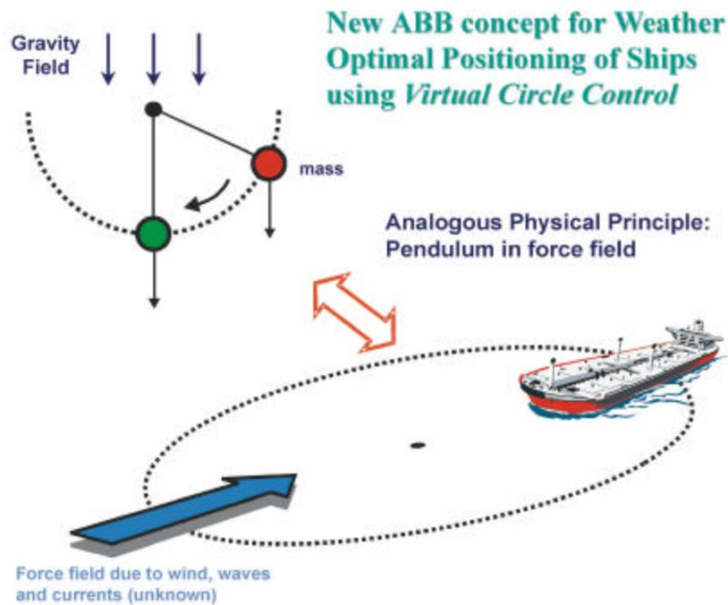
**Figure 3.** Analogy between a pendulum in the gravity field and weather optimal positioning.
