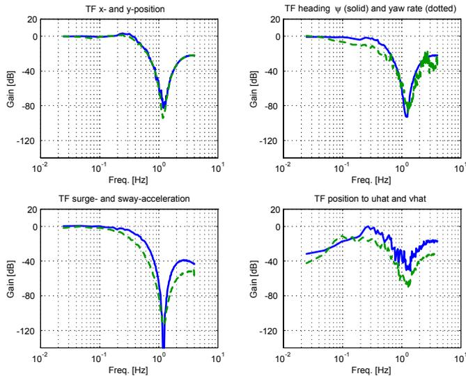
Figure 6: Top left, TF from measured North (solid) and East (dotted) position to their respective LF estimates. Top right, TF from measured heading (solid) and yaw rate (dotted) to LF estimates. Bottom left, TF from measured surge (solid) and sway acceleration to LF estimates. Bottom right, TF from North position to surge velocity (solid) and from East to sway (dotted).
