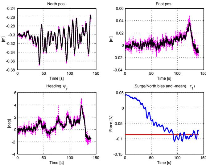
Figure 4: Top left, measured (dotted) and LF estimated North position. Top right, measured (dotted) and LF estimated East position. Bottom left, measured (dotted) and LF estimated heading. Bottom right, estimated bias and mean of applied thrust  $\tau_1$ .
