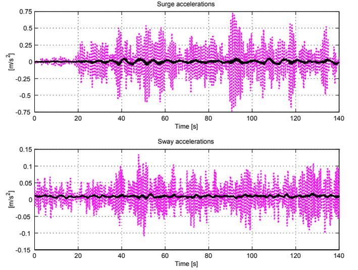
Figure 5:  $g$ -compensated surge and sway accelerations. Measurements (dotted) and LF estimates (solid).
