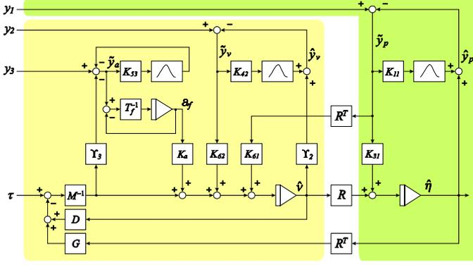
Figure 1: Observer with first order cut-off filter for acceleration. Bias estimation is not shown.
