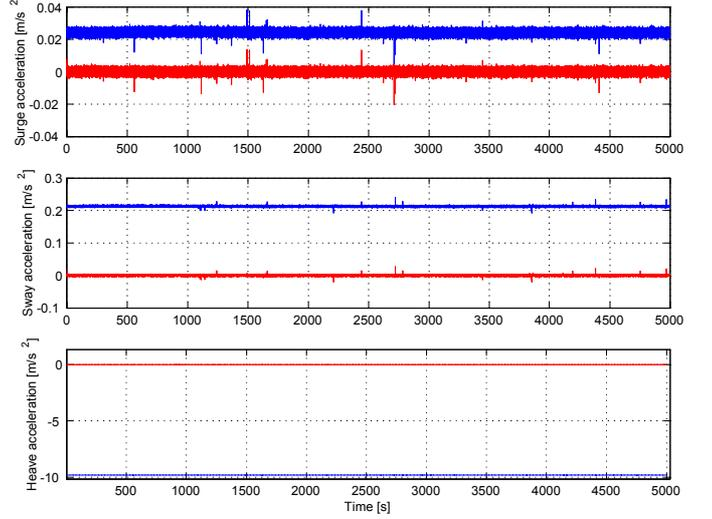
Figure 2: Measured and g-compensated accelerations. The noise level is about 120  $\mu g$  ( $1\sigma$ ), and the offset after compensation is a few  $\mu g$  on all three axes.
