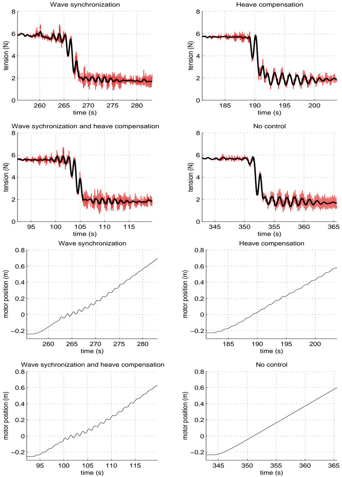
Fig. 7. Experimental results with regular waves at  $T = 1.25$  s and  $A = 1.8$  cm, spherical payload, test B. For the wire tension we show both raw data (thin lines) and low-pass filtered data (thick lines). The payload position (measured using the motor shaft encoder) is in a vessel-fixed coordinate frame, with zero at mean sea level.
