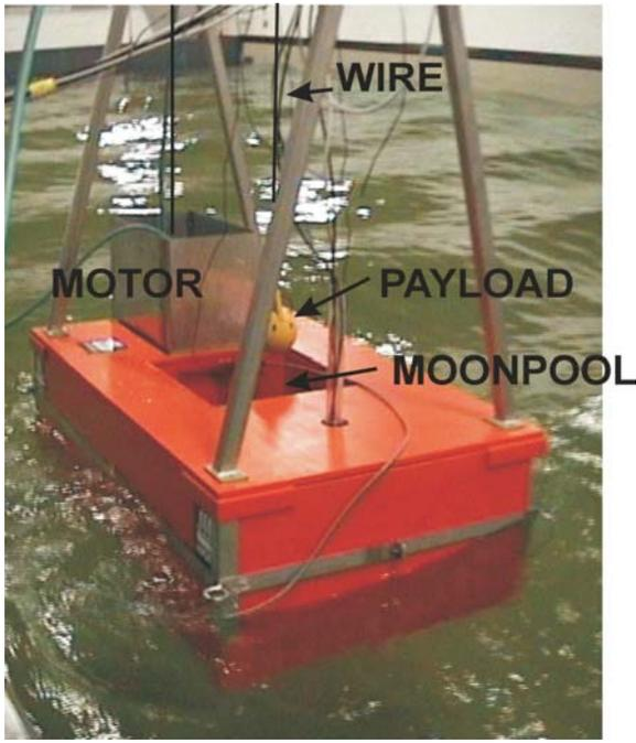
Fig. 1. Vessel-crane scale model.
