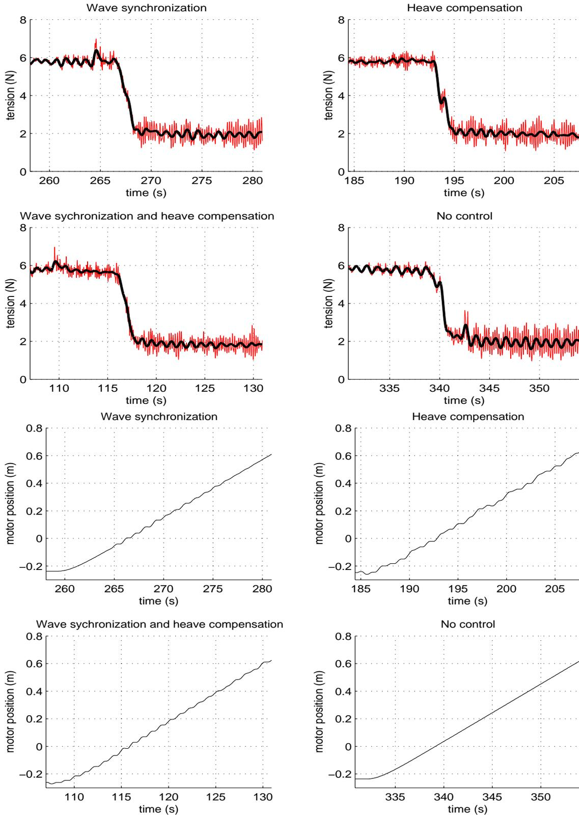
Fig. 8. Experimental results with regular waves at  $T = 1.00$  s and  $A = 6.8$  cm, spherical payload, test B. For the wire tension we show both raw data (thin lines) and low-pass filtered data (thick lines). The payload position (measured using the motor shaft encoder) is in a vessel-fixed coordinate frame, with zero at mean sea level.
