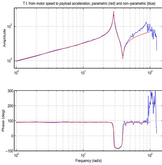
Fig. 4. Parametric and spectral estimates of the transfer function  $\ddot{z}/\dot{\omega}_m(s)$ .
