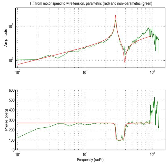
Fig. 5. Parametric and spectral estimates of the transfer function  $F_t/\dot{\omega}_m(s)$ .
