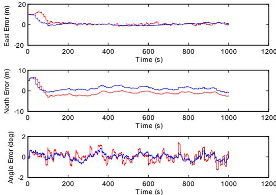
Fig. 5. Estimation errors of the EKF (dark line) and the LMI estimator (light line) for the straight line case.
