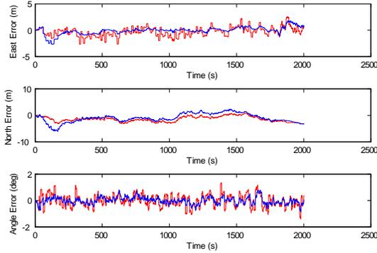
Fig. 8. Estimation errors of the EKF (dark line) and the LMI estimator (light line) in the lawn-mowing maneuver.
