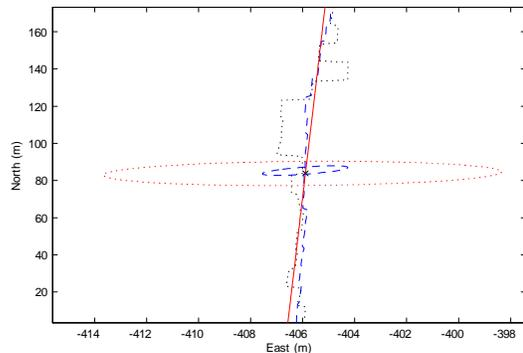
Fig. 7. Zoom to a portion of the lawn-mowing maneuver. The true value is signaled with a cross, the confidence ellipsoids of the EKF and the LMI observer are dashed and dotted respectively.
