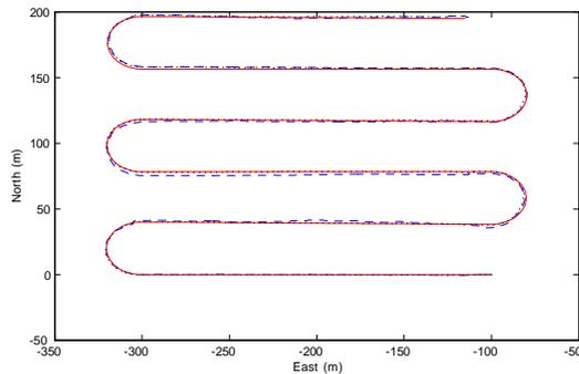
Fig. 9. Simulated lawn-mowing trajectory with some bad measurements. The solid line is the real trajectory and the dashed and dotted lines are the EKF and the LMI observer estimations.
