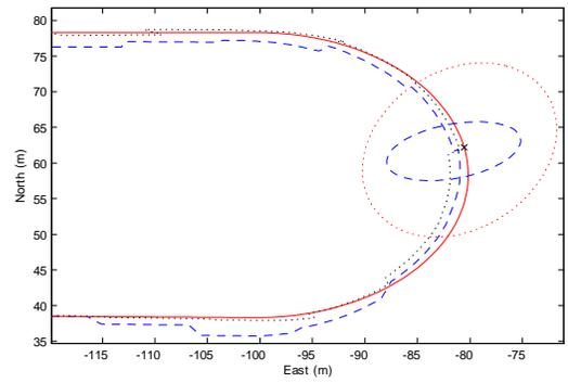
Fig. 11. Zoom to a portion of the lawn-mowing maneuver where some bad measurements affected the estimation; the true value is signaled with a cross, the confidence ellipsoids of the EKF and the LMI observer are dashed and dotted respectively.
