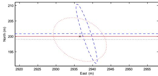
Fig. 4. Confidence region for both filters. The cross is the real position, while the dashed and dotted ellipsoids are the EKF and the LMI observer regions of confidence.
