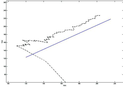
Fig. 2. Estimate (dotted) and true (solid) trajectories. Due to the noise and to the proximity of the points that satisfy the measurement equation the estimate may not be correct.
