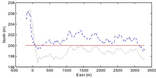
Fig. 3. Simulated straight line trajectory. The solid line is the real trajectory and the dashed and dotted lines are the EKF and the LMI observer estimations.
