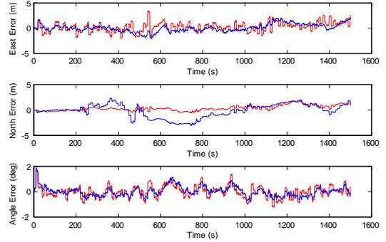
Fig. 10. Estimation errors of the EKF (dark line) and the LMI estimator (light line) in the lawn-mowing maneuver with non-Gaussian noise during a period of time.
