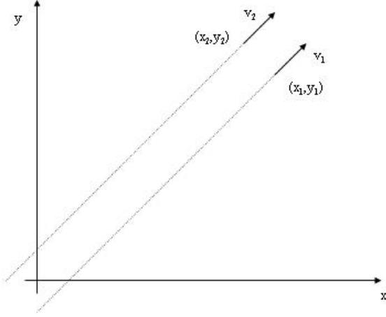
Fig. 1. Two indistinguishable trajectories. The yaw angle and the distance to the transponder are equal in both cases at each time sample.
