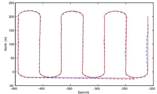
Fig. 6. Simulated lawn-mowing trajectory. The solid line is the real trajectory and the dashed and dotted lines are the EKF and the LMI observer estimations.
