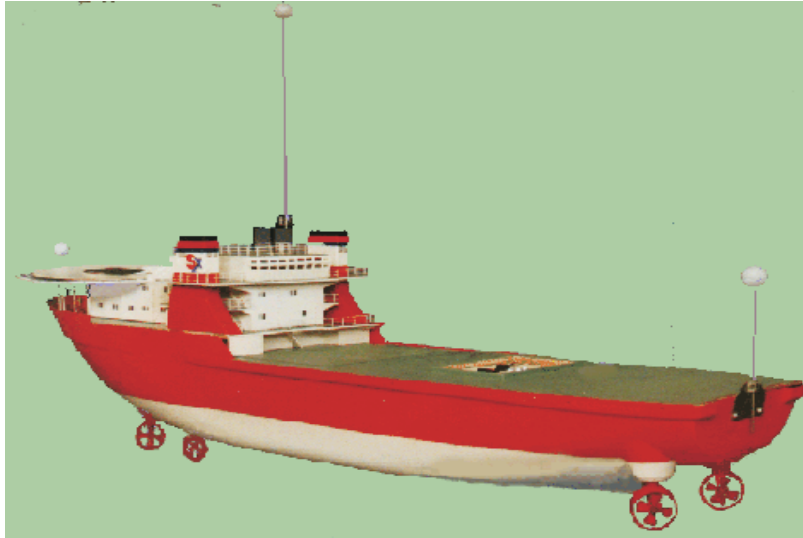
Fig. 2. Picture of Cybership I, a 1:70 scale model of a supply ship with 4 azimuth thrusters.
