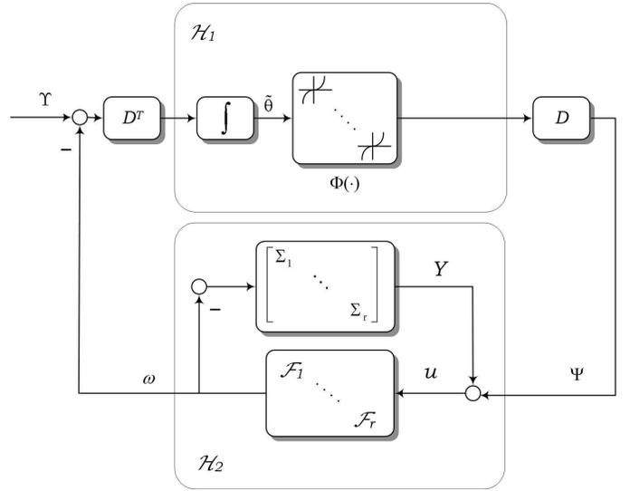
Fig. 1. Block diagram for the synchronized path following control system.  $\Upsilon$  is a  $r \times 1$  vector with each entry equal to  $v(t)$ .
