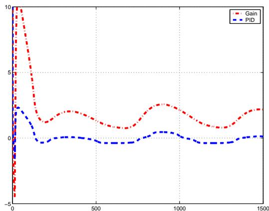
Fig. 6. Synchronization of  $\tilde{\theta}_1$  when one vessel saturates. The result when  $\mathcal{F}_i$  is a gain is shown in red (dashed-dot) and a PID structure for  $\mathcal{F}_i$  results in the blue (dashed) plot.
