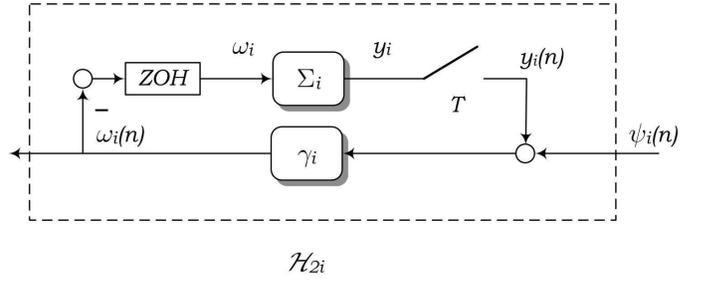
Fig. 3. A block diagram representation of the sampled-data dynamical block  $\mathcal{H}_{2i}$  where ZOH stands for the "Zero-Order-Hold" function and  $T$  is the sampling period.
