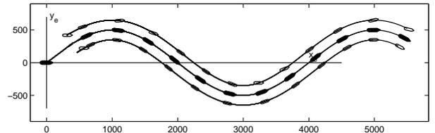
Fig. 5. Position snapshots of three tugboats where one vessel saturates. The feedback function  $\mathcal{F}_i$  is as in (55).
