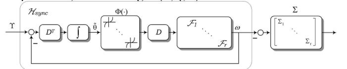
Fig. 2. Cascade interconnection for Design 2.
