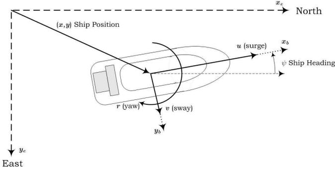
Fig. 4. Earth-fixed and body-fixed reference frame for a ship.
