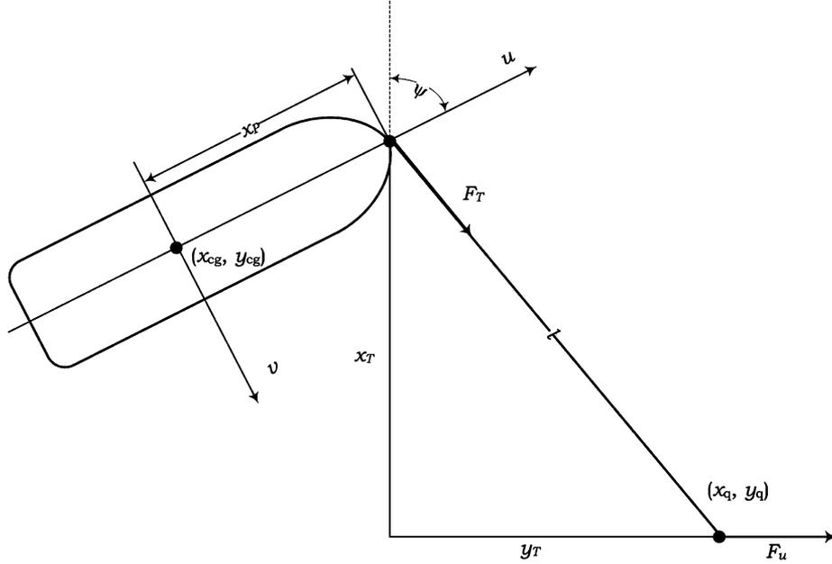
Fig. 3. Point mass and underactuated vessel.
