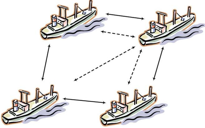
Fig. 2. Different constraint functions acting between vessels determine collective motion. Two types of constraint functions are illustrated:  $C_{rd}$  (—) and  $C_{fd}$  (---).
