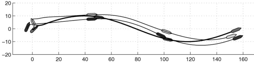
Fig. 8. Position plot of the three vessels in a constrained formation during trajectory tracking. The bold line is vessel 1 following the desired trajectory  $\eta_d(t)$ .
