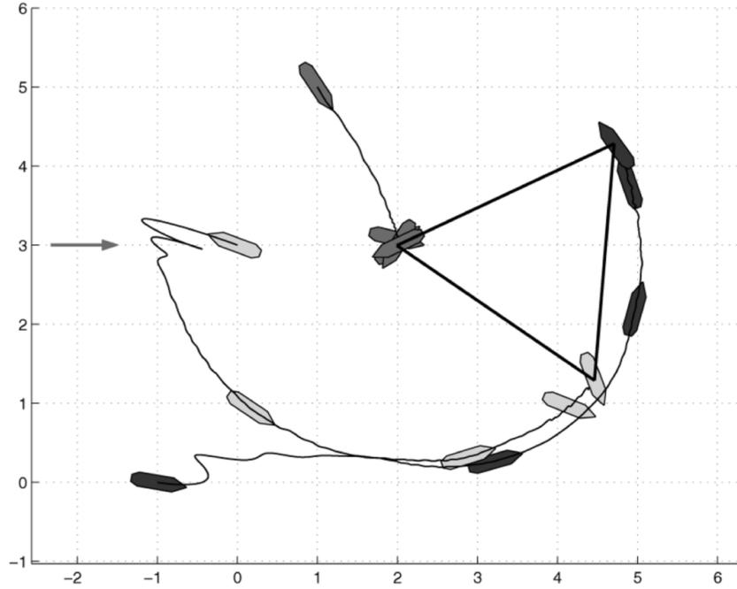
Fig. 6. Position of vessels during assembling while vessel 1 is positioned at  $\eta_{\text{des}} = [2, 3, 0]^T$ . The arrow is the unknown bias. Final configuration is shown as a solid line.
