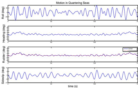
Fig. 3. Motion of the vessel in quartering seas ( $\chi=60$  deg). ITTC Spectrum:  $H_s=2$ m,  $t_0=9$ s
