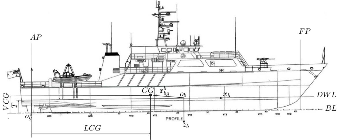
Fig. A.1. Vessel profile and reference frames. Reproduced with permission of ADI-limited Australia.
