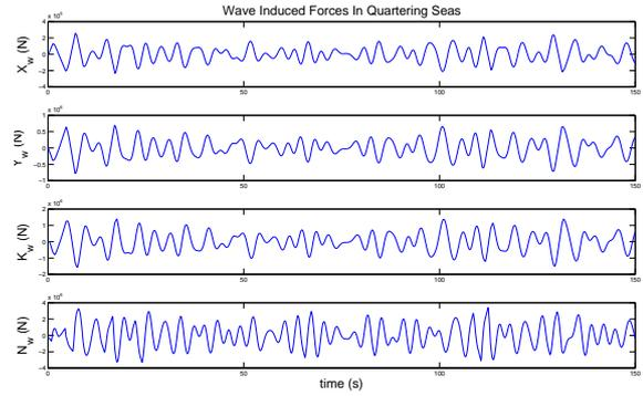
Fig. 4. Wave induced forces on the vessel in quartering seas ( $\chi=60$  deg). ITTC Spectrum:  $H_s=2$  m,  $t_0=9$  s
