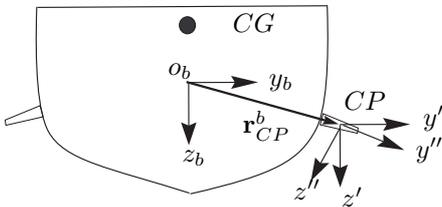
Fig. 1. Reference frames used to compute fin forces.
