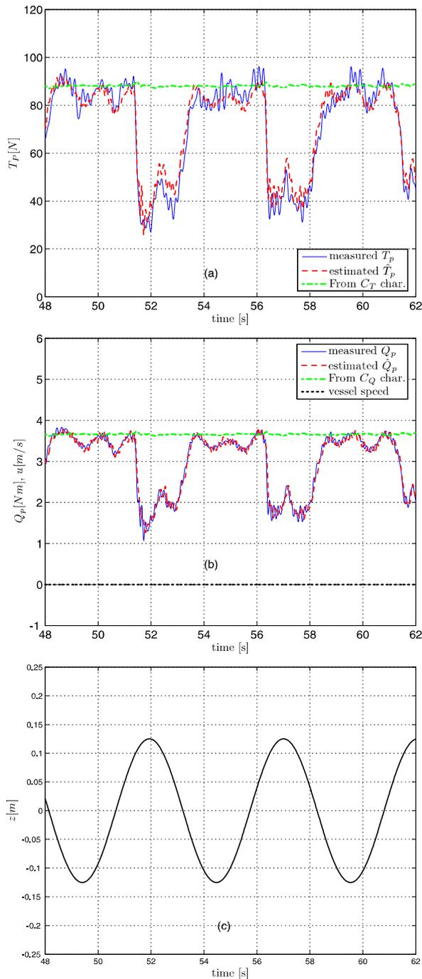
Fig. 10. Experimental results with waves and constant shaft speed.
