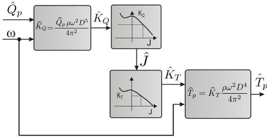
Fig. 5. Thrust estimation block diagram.
