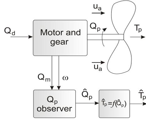
Fig. 2. Propeller thrust estimation scheme.
