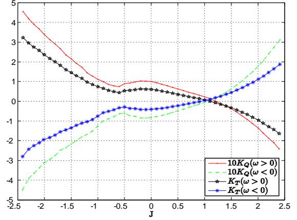
Fig. 3. Propeller characteristics  $K_T$  and  $K_Q$ .
