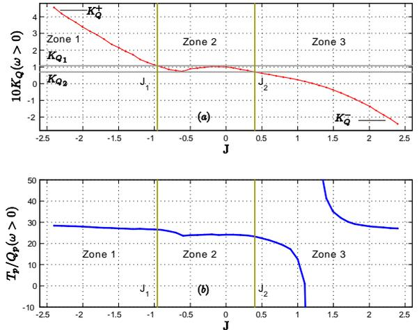
Fig. 4.  $K_Q$  characteristic and the ratio between thrust and torque for  $\omega > 0$ .
