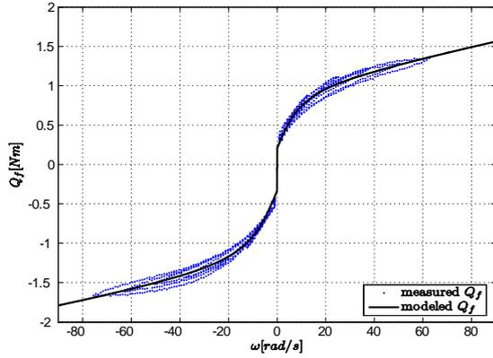
Fig. 8. Friction torque: computed from measurements and a static approximation.
