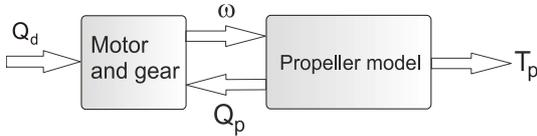
Fig. 1. Propeller system block diagram.
