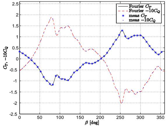
Fig. 7. Propeller four-quadrant open water characteristics.
