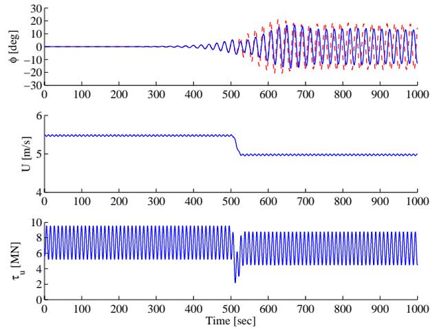
Fig. 3. Stabilisation of roll angle  $\phi$  with only speed controller active. Roll in parametric resonance (red dashed curve)
