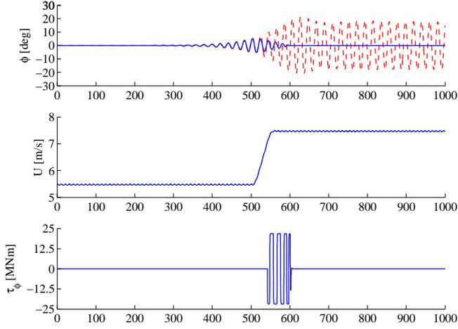
Fig. 4. Stabilisation of roll angle  $\phi$  using the plant model ( $\Delta U = 2$  m/s,  $\tau_{\phi, \max} = 21.8$  MNm). Roll in parametric resonance (red dashed curve)
