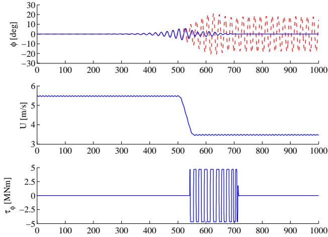
Fig. 5. Stabilisation of roll angle  $\phi$  using the plant model ( $\Delta U = -2$  m/s,  $\tau_{\phi, \max} = 4.7$  MNm). Roll in parametric resonance (red dashed curve)
