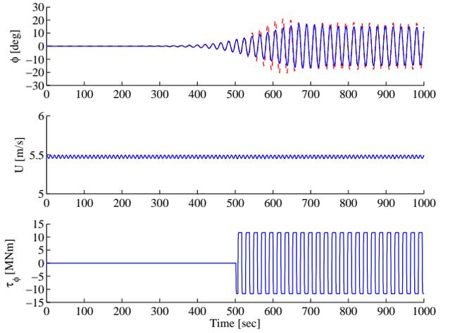
Fig. 2. Stabilisation of roll angle  $\phi$  with only fin stabiliser active. Roll in parametric resonance (red dashed curve)
