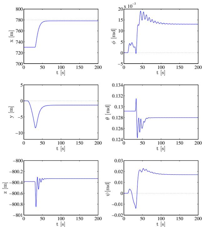
Fig. 3. Postion and orientation of  $\eta$  over the course of the simulation. The PD-controller is enabled at  $t = 30s$ . The dotted line indicates  $\eta_{ref}$  for the controlled states. Note the bias.
