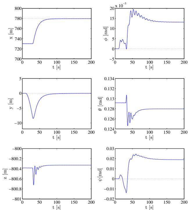
Fig. 4. Postion and orientation of  $\eta$  over the course of the simulation. The PID-controller is enabled at  $t = 30s$ . The dotted line indicates  $\eta_{ref}$  for the controlled states. Note that the integrator term cancels the bias terms seen when the PD-controller was applied.
