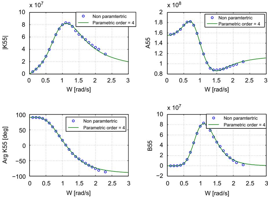
Fig. 3. Results of a 4th-order parametric approximation of the convolution term in pitch.
