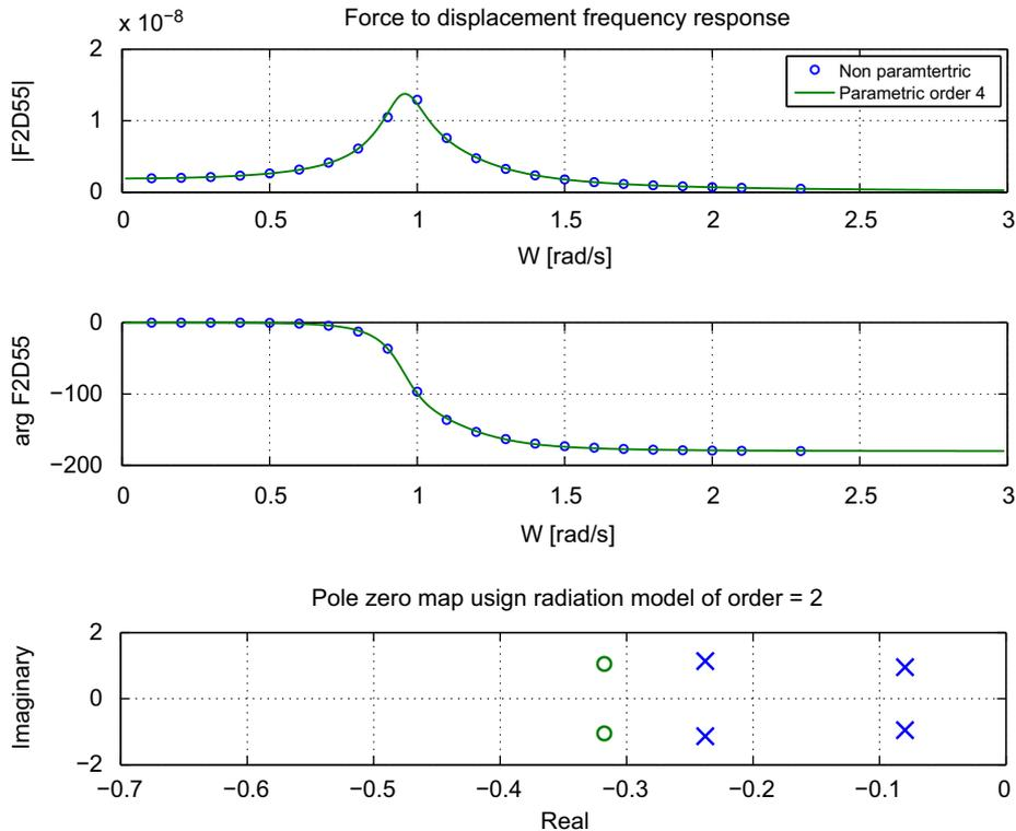
Fig. 9. Force-to-displacement frequency response function and pole-zero map corresponding to a 2nd-order parametric approximation of the convolution term.
