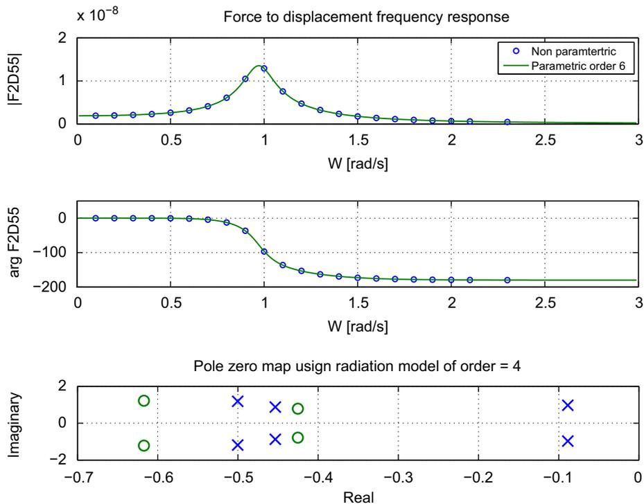
Fig. 5. Force-to-displacement frequency response function and pole-zero map corresponding to a 4th-order parametric approximation of the convolution term.
