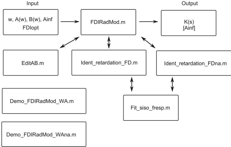
Fig. 2. Organisation of the MSS-FDI toolbox for frequency-domain identification of radiation models of marine structures ([www.marinecontrol.org](http://www.marinecontrol.org)).
