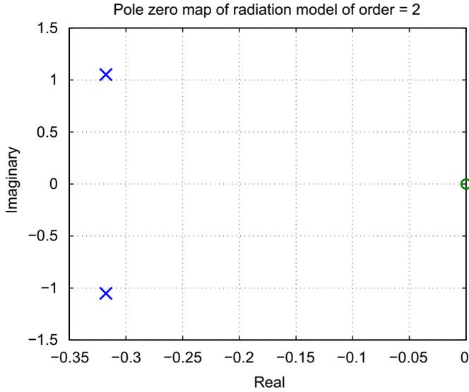
Fig. 8. Pole-zero map of the 2nd-order parametric approximation of the convolution term in pitch.
