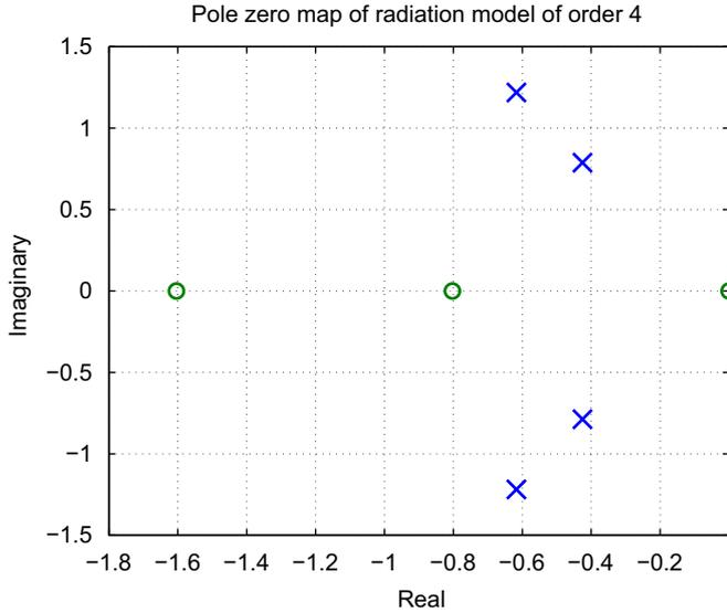
Fig. 4. Pole-zero map of the 4th-order parametric approximation of the convolution term in pitch.
