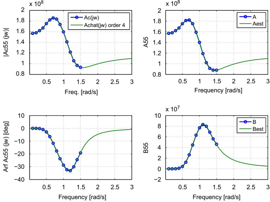
Fig. 6. Results of a 4th-order parametric approximation for joint convolution and infinite-frequency added mass estimation.
