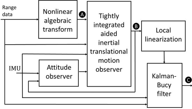
Fig. 2. Final-stage estimation using the linearized Kalman-Bucy filter. Position and velocity estimates are output with increasing accuracy at outputs A, B, and C, respectively.
