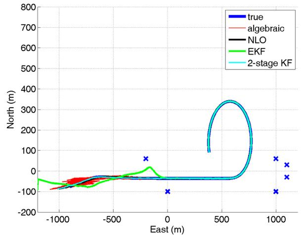
Fig. 3. Horizontal position estimated with different observers. The initial position is at -1100 m East and -80 m North. The six beacon positions are marked by blue points.
