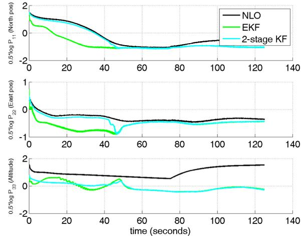
Fig. 6. Square root of the diagonal elements of covariance matrices corresponding to position estimates. Note the logarithmic scale.
