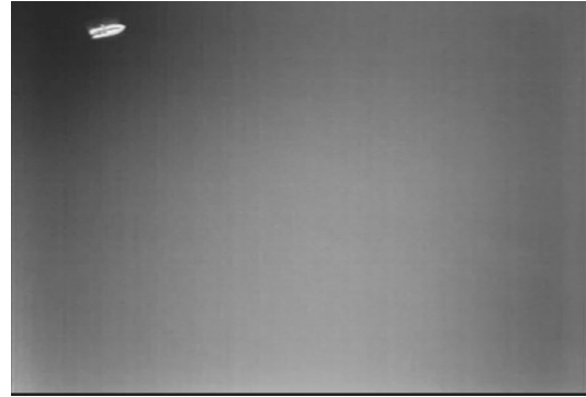
Fig. 5 A thermal image captured at the flight experiment. A small boat is present in the image.
